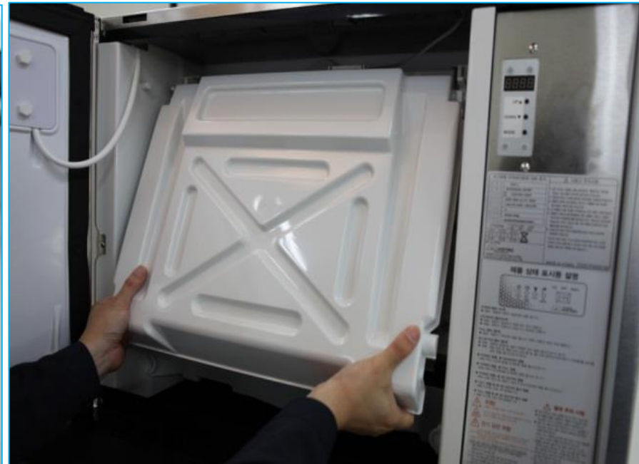
PULL CURTAIN OPEN ABOUT 30 DEGREES LIFT & PULL FORWARD TO REMOVE
