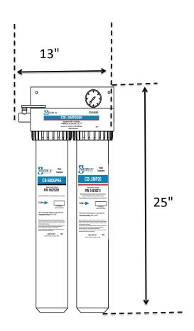
All carbon block cartridges should be changed out every six months or when there is a reduction in water pressure. Filter life depends greatly upon the quality of water. This product is for commercial use only and must be installed and maintained according to manufacturers guidelines www.systemsiv.com or the warranty can be voided.
